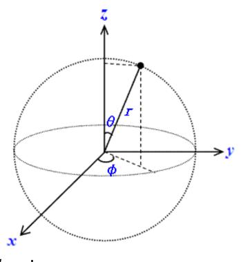
$$\left| \frac{\partial \vec{r}}{\partial \theta} \times \frac{\partial \vec{r}}{\partial \varphi} \right| = r^2 \sqrt{\sin^4 \theta \cos^2 \varphi + \sin^4 \theta \sin^2 \varphi + \sin^2 \theta \cos^2 \theta}$$
