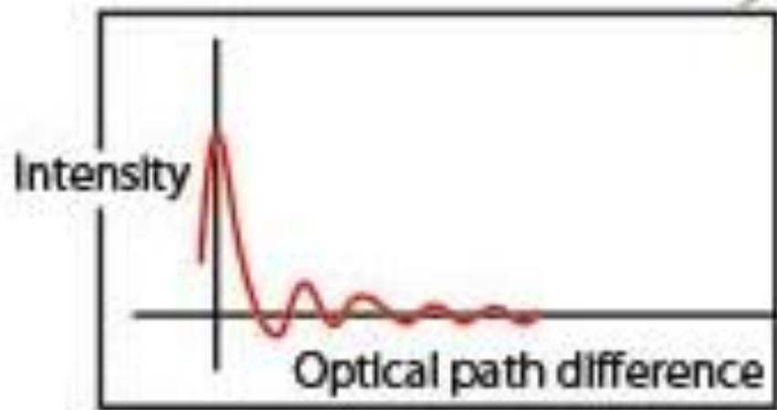
Signal of Interference Wave
